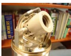
DOR probe built by the group of David Bryce (Ottawa University). Typical spinning rate is 1.5 kHz for the outer rotor and 7 kHz for the inner rotor.
