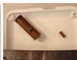
DOR probe built by the group of David Bryce (Ottawa University). Typical spinning rate is 1.5 kHz for the outer rotor and 7 kHz for the inner rotor.
